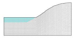
Set up a cross section with a lake represented by  $K = 0.01 \text{ m s}^{-1}$ .
